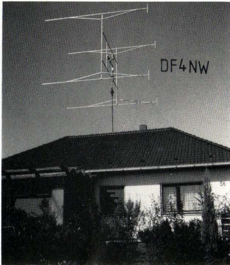
Fig. 7: The author's 4 x 17-el. Yagi, EME array.
