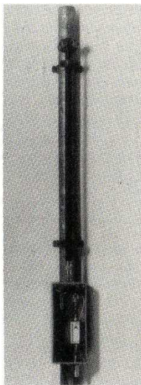
Fig. 8: The pre-amplifier/ relay unit from fig. 5 affixed to a coaxial matching trans- former
