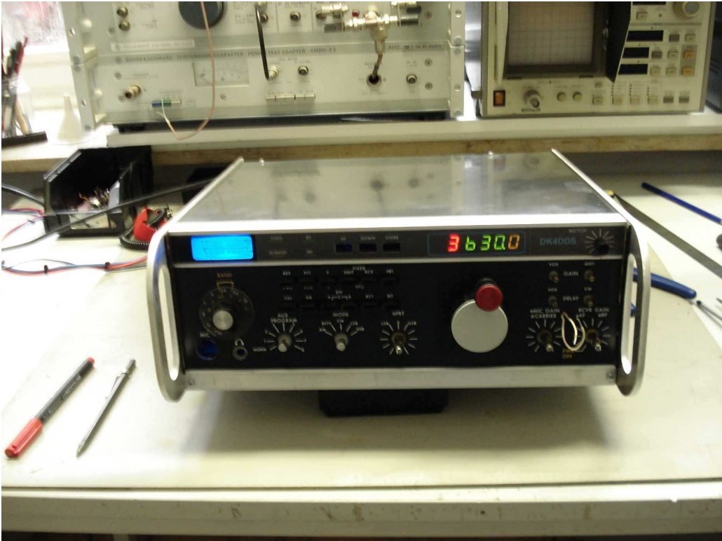
Marc's new version of a modernised and modified TR7 with multicolour frequency display and the PTO replaced by a DDS VFO.
